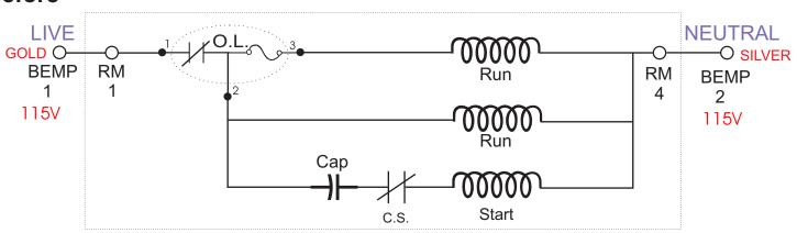
The RED and BLUE wires of the Solid State Start Switch take the place of the mechanical start switch.
